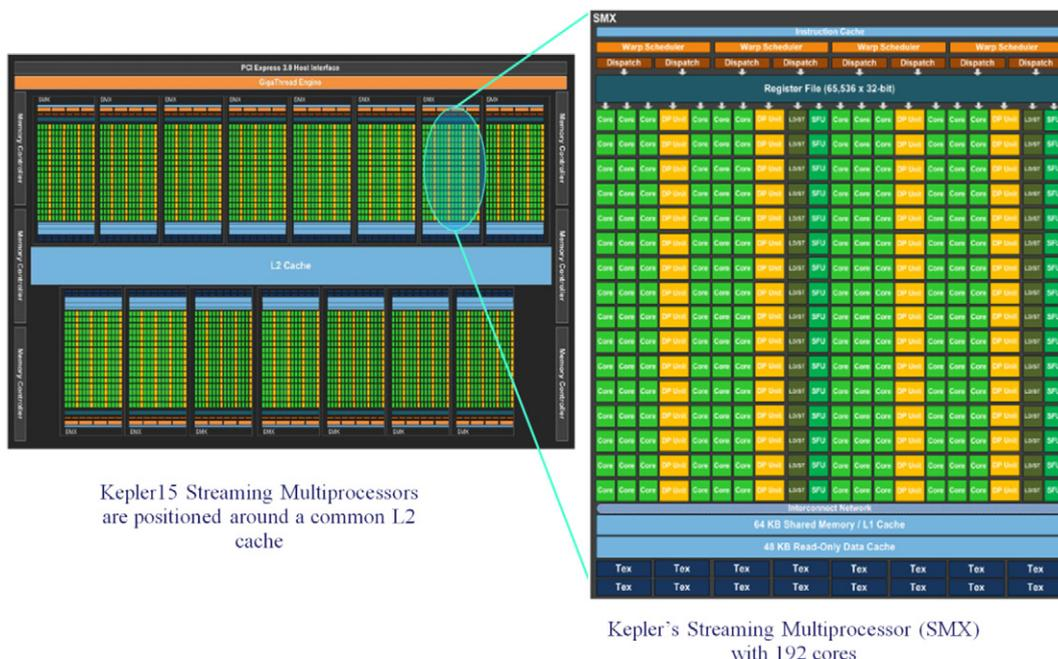
Kepler15 Streaming Multiprocessors are positioned around a common L2 cache
